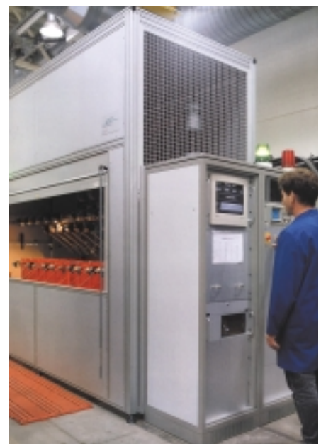
Automized routine test facility for Metal-Oxide Surge Arresters in the manufacturing area in Ottobrunn/Munich, Germany
