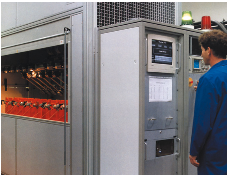
Automated routine test facility for Metal-Oxide Surge Arresters in the manufacturing area
